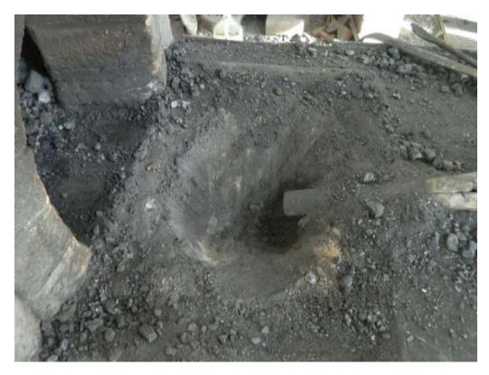
This setup needs to be altered a little to make steel and forge with charcoal, since my bin that holds the ash is a little too shallow for this. I need at least 3 inches below the tuyere to make a carburizing zone, as in the
