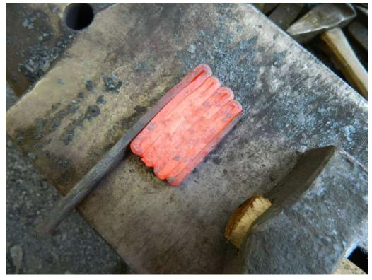
... and spread it a little with a chisel tip so carbon monoxide can get at all the surfaces...
