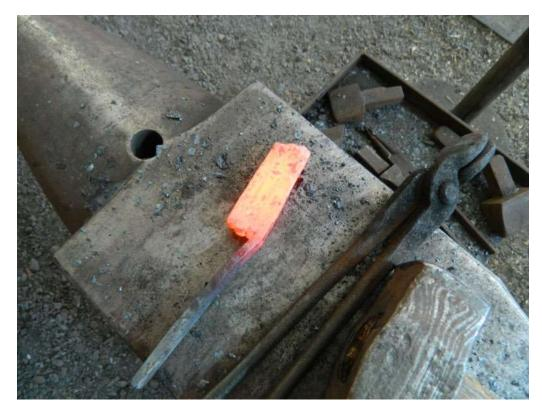
On a billet I remembered to weigh, the accordion weighed 360 grams at accordion stage, and 280 grams after carburizing and welding.
