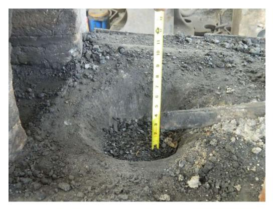
Then I need some walls to contain the charcoal. In this case, I've just piled up some bricks, two walls of clay would be the tidier and more traditional option. The carburizing zone will be <u>below the tuyere</u>, on this floor of charcoal fines.
