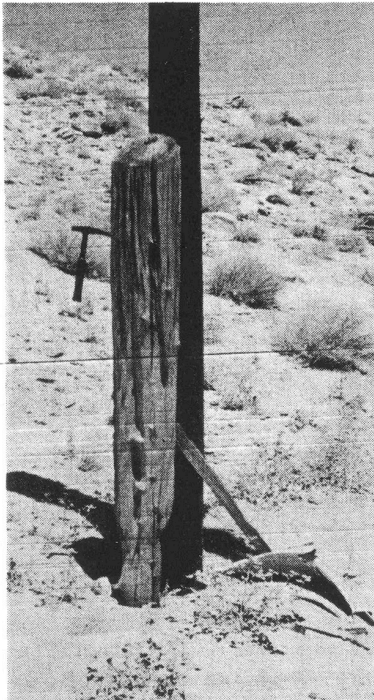
BY COURTESY OF H. T. U. SMITH WIND EROSION ON A WOODEN POLE USED AS A BUFFER TO PROTECT THE POLE BEHIND IT
