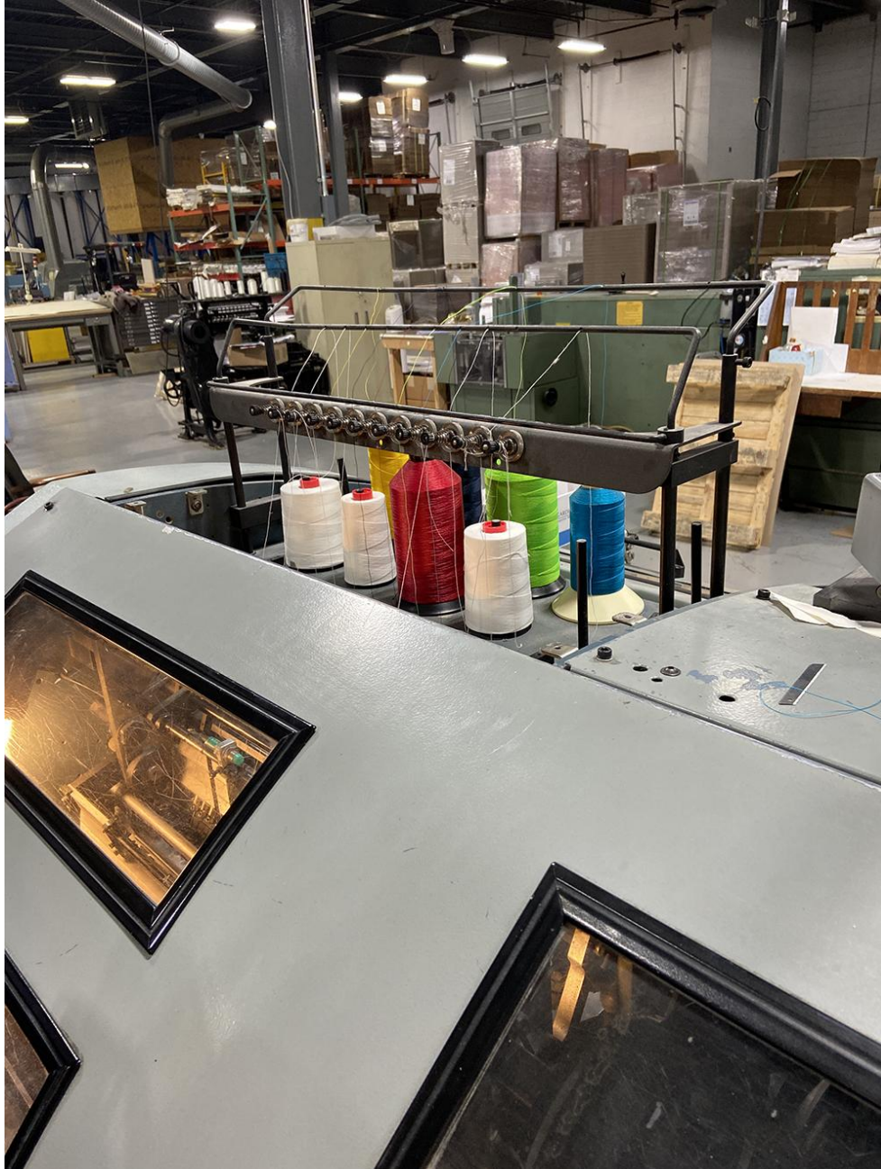
Smyth Sewn binding machine with colored threads selected for The Garden at Bassil Bookbinding, Co., Hackensack, NJ, January 2022.
