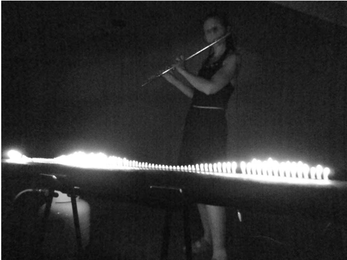
FIG. 2 – A Rubin's Tube is a simple apparatus used to make sound waves visible in flames. Here I am manipulating a row of flames using sounds produced by an amplified flute.
